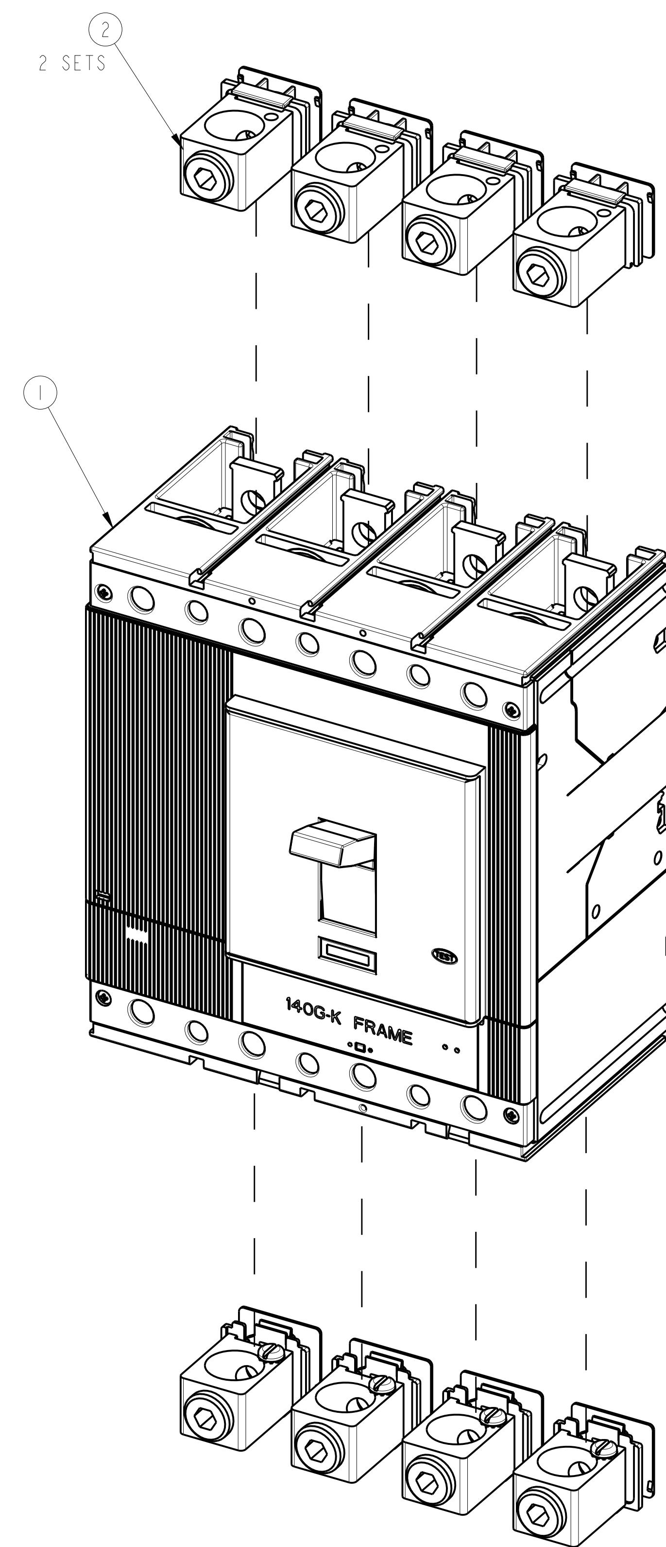
TERMINAL FOR FCCU ASSEMBLED TO 140G-K-4-POLE
