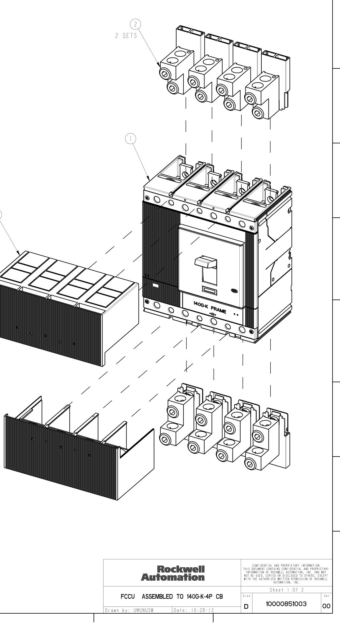
TERMINAL FOR ASSEMBLED TO 140G-K-4-POLE SCALE 0.6:I
