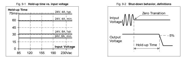
Note: At no load, the hold-up time can be up to one minute. The green DC-ok lamp is on during this time.
