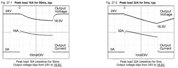
Please note: The DC-OK relay triggers when the voltage dips more than 10% for longer than 1ms.
