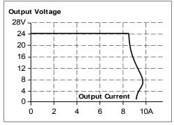
The Power-Boost is available as soon as power comes on and immediately after the end of an output short circuit.
