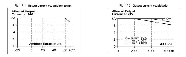
The ambient temperature is defined as the air temperature 2cm below the unit.
