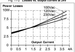
Fig. 11-4 Losses vs. input voltage, 24V, 3.8A
