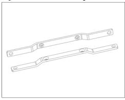
Fig. 26-2 Assembled Wall Mounting Bracket
