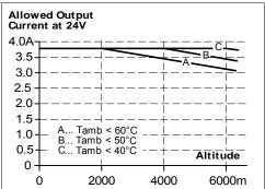
The ambient temperature is defined as the air temperature 2cm below the unit.
