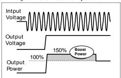
Fig. 8-3 Power-Boost after output short
