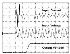
Input: 230Vac Output: 24V, 3.8A Ambient: 25°C
