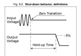
Note: At no load, the hold-up time can be up to one minute. The green DC-ok lamp is on during this time.
