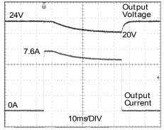
Peak load 7.6A (resistive) for 50ms Output voltage dips from 24V to 20V.
