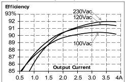
Fig. 11-3 Efficiency vs. input voltage, 24V, 3.8A
