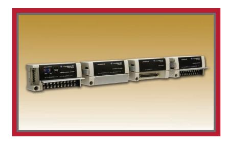
CompactBlock™ LDX I/O is a compact, cost-effective, and diverse distributed I/O solution for light industrial and commercial automation environments. Offering 24 VDC, 120 VAC, relay, analog, and temperature blocks, CompactBlock LDX supports a wide range of field devices and is compatible on both DeviceNet™ and PROFIBUS® DP.
