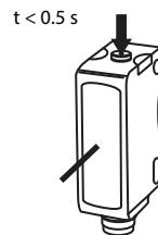
Press and release the button within ten seconds to toggle from L.O. to D.O., the selection indicated by the yellow LED.
