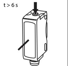
Press and hold button for six seconds until the green LED starts flashing. Release the button. The current setting is indicated by the yellow LED:
