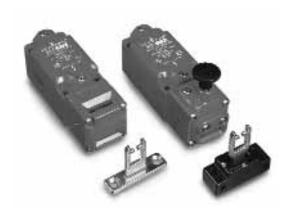
The MT-GD2 family is a robust, tongue-operated (or key-operated) safety-interlock switch designed to fit at the leading edge of sliding, hinged or lift-off guards. With its dual entry slots and rotatable head, the MT-GD2 can offer eight different options for actuator entry.
