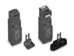
The Cadet 3 is a tongue-operated (or key-operated) safety interlock switch designed to fit at the leading edge of sliding, hinged or lift-off guards. With its dual entry slots and rotatable head, the versatile Cadet 3 can offer up to eight different actuator entry options. The unique compact housing (90.5 x 31 x 30.4 mm (3.56 x 1.22 x 1.19 in)) has industry standard DIN 50047 fixing centers for ease of mounting.
