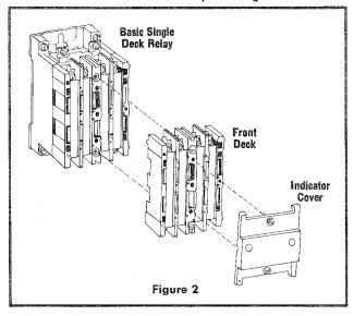
**ADDING TIMER** — The Bulletin 852S Solid State Timer can be added to any single deck relay. Do not remove the cover of the single deck relay. Remove mounting plate
