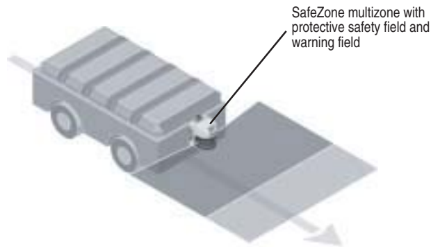
Figure 56: Vehicle monitoring with SafeZone safety laser scanner
