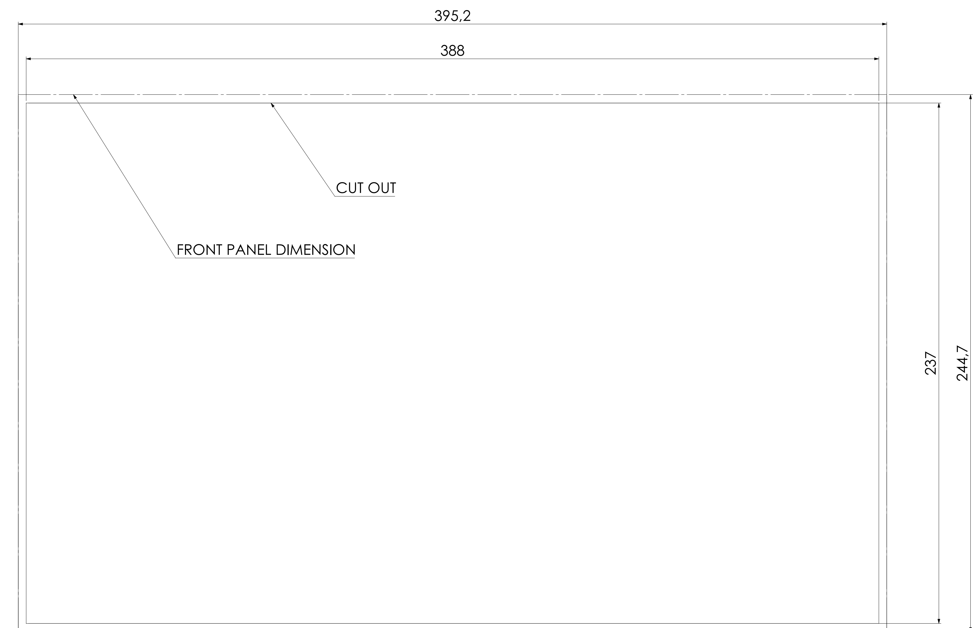
VersaView 6300P (Fanless) 6300P-156AAPSFDB 15.6" Inch Display dimensions are in mm
